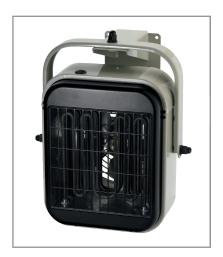
The thermal protector automatically disconnects the unit in the case of overheating. They have a manual RESET button, situated at the top of the housing to reconnect the unit. They also have a switch that allows the thermostat to act on both the fan and the heater element or only on the heater.
